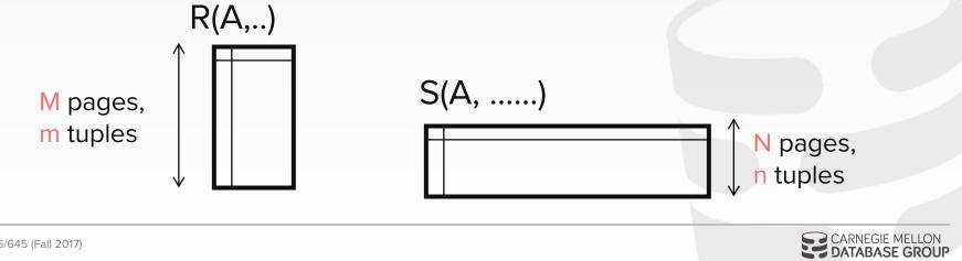
This algorithm uses B-2 buffers for scanning M. Number of disk accesses  $\rightarrow$  Cost: M + ( $\lceil M/(B-2) \rceil \cdot N$ )
