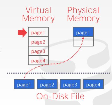
One can use memory mapping (mmap) to store the contents of a file into a process' address space.
