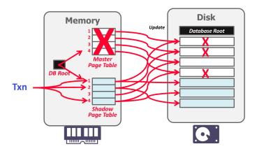
**Figure 2: Shadow Paging** – The database root points to a master page table which points to the pages on disk. When an updating transaction occurs, a shadow page table is created that points to the same pages as the master. Modifications are made to a temporary space on disk and the shadow table is updated. To commit, the database root pointer is redirected to the shadow table, which becomes the new master.
