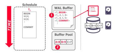
**Figure 3:** Write Ahead Logging – When the transaction begins, all changes are recorded in the WAL buffer in memory before being made to the buffer pool. When it comes time to commit, the WAL buffer is flushed out to disk. The transaction result can be written once the WAL buffer is safely on disk.
