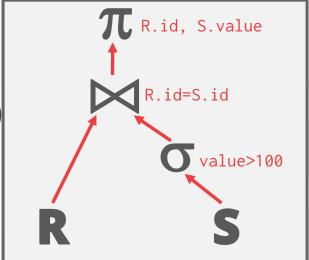
This is used in almost every DBMS. Allows for tuple pipelining.
