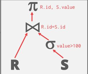
for t in child.Next(): emit(projection(t)) for t<sub>1</sub> in left.Next(): buildHashTable(t<sub>1</sub>) for t₂ in right.Next()← if probe(t):  $emit(t_1 \bowtie t_2)$ for t in child.Next(): if evalPred(t): femit(t) for t in R: for t in \$ emit(t) emit(t)
