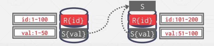
Both tables are partitioned on different keys. If one of the tables is small, then the DBMS "broadcasts" that table to all nodes.
