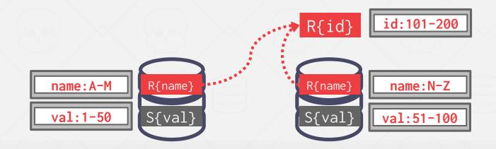
Both tables are <u>not</u> partitioned on the join key. The DBMS copies the tables by "shuffling" them across nodes.
