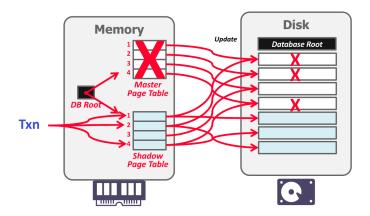
**Figure 2: Shadow Paging** – The database root points to a master page table which in turn points to the pages on disk (all of which contain committed data). When an updating transaction occurs, a shadow page table is created that points to the same pages as the master. Modifications are made to a temporary space on disk and the shadow table is updated. To complete the commit, the database root pointer is redirected to the shadow table, which becomes the new master.
