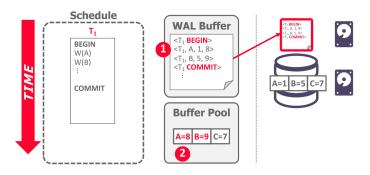
**Figure 3:** Write Ahead Logging – When the transaction begins, all changes are recorded in the WAL buffer in memory before being made to the buffer pool. At the time of commit, the WAL buffer is flushed out to disk. The transaction result can be written out to disk, once the WAL buffer is safely on disk.
