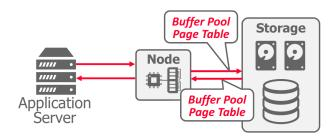
**Figure 3: Serverless Database** – When the application server becomes idle, the user must pay for resources in the node that are not being used. In a serverless database, when the application server stops, the DBMS takes a snapshot of pages in the buffer pool and writes it out to shared disk so that the computation can be stopped. When the application server returns, the buffer pool page table restores the previous state in the node.
