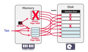
**Figure 2: Shadow Paging** – The database root points to a master page table which in turn points to the pages on disk (all of which contain committed data). When an updating transaction occurs, a shadow page table is created that points to the same pages as the master. Modifications are made to a temporary space on disk and the shadow table is updated. To complete the commit, the database root pointer is redirected to the shadow table, which becomes the new master.
