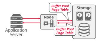
**Figure 3: Serverless Database** – When the application server becomes idle, the user must pay for resources in the node that are not being used. In a serverless database, when the application server stops, the DBMS takes a snapshot of pages in the buffer pool and writes it out to shared disk so that the computation can be stopped. When the application server returns, the buffer pool page table restores the previous state in the node.
